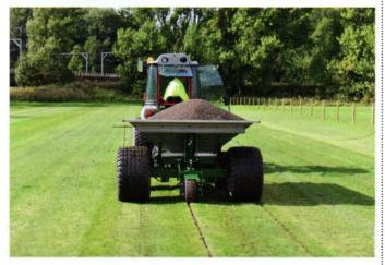
"Air injection systems, such as the Gwazae, push air in under force and break up compacted soil. Because the surface is hardly disturbed, it can be a good way of treating fine sportsturf areas like golf greens, around goalmouths and under racecourse jumps."
