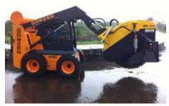
This compact trencher is designed to be mounted onto skid steer loaders with a "high flow" option. The combination of heavy duty trencher and loader is the ideal solution for fast and tidy trenching in difficult conditions where access is limited. It will cut the narrowest of trenches even when trenching in concrete
